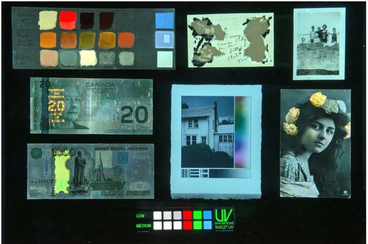
Examples of fluorescent attributes in currency, photographs and a common range of paints and pigments. The UV Innovations™ standard, developed at the studio for repeatable and interoperable UV imaging, is seen below. © Jiuan Jiuan Chen, Paul Messier LLC
