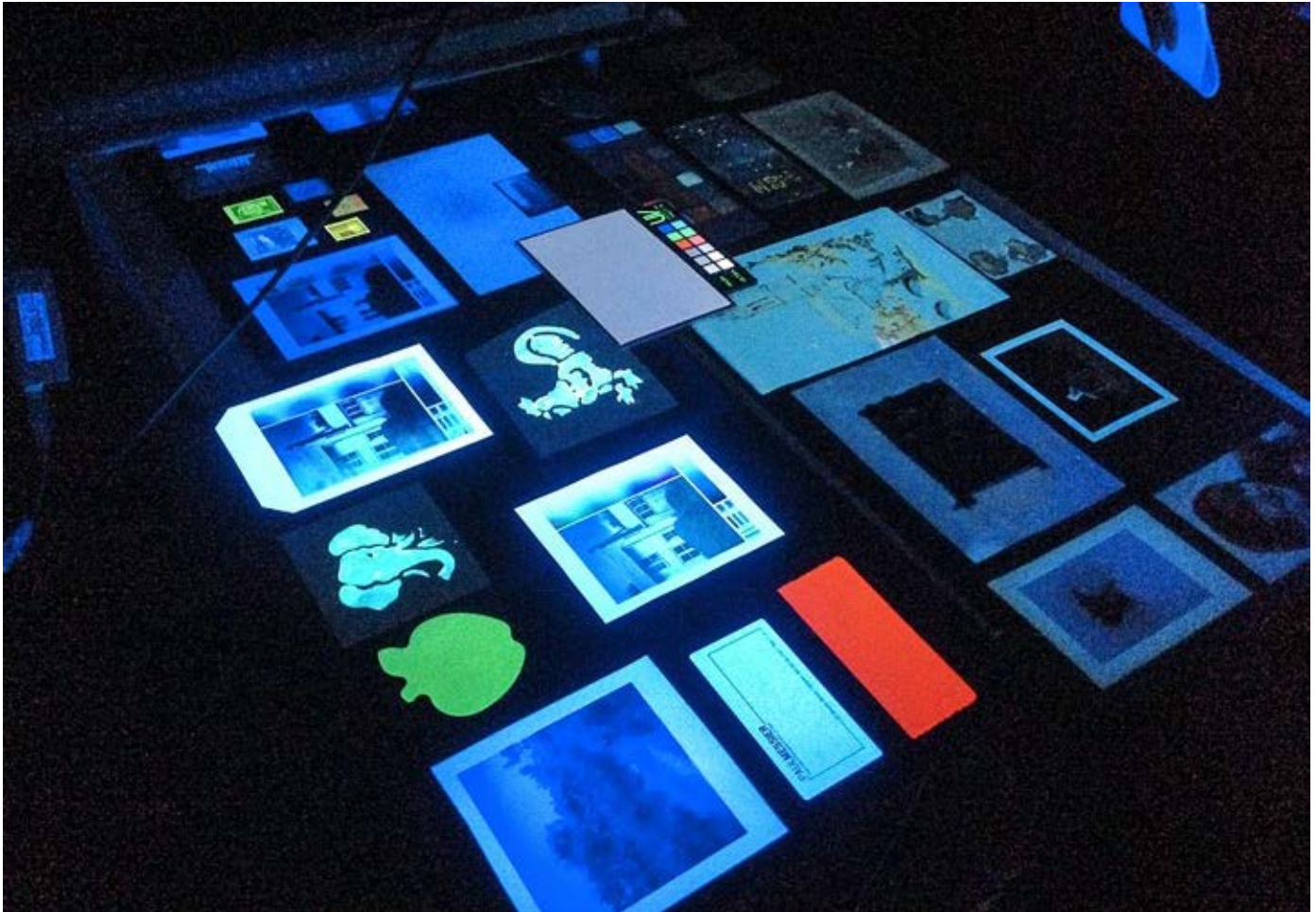
Various photographic media viewed under UV, showing the range of fluorescent intensities and colours. Since the Lewis Hine research, the studio has made significant strides in the use of UV as a tool to investigate the condition and material history of photographs. © Juan Juan Chen, Paul Messier LLC
